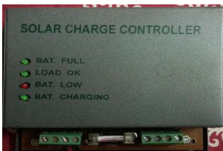
Fig.5. Solar Charge controller
