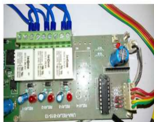
Fig 14:Circuit showing Darlington amplifier used in project.
