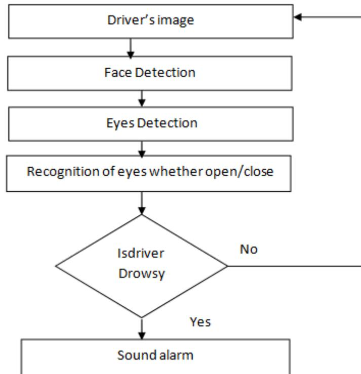
Figure 1. System Flow Diagram
