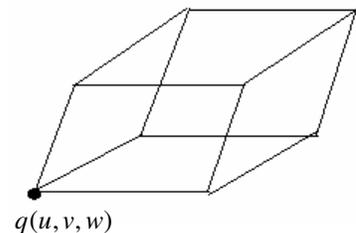
The edges which are considered as arcs will be taken as  $\lambda\delta\alpha$ ,  $\mu\delta\beta$  and  $\nu\delta y$ . Here,  $\lambda, \mu, \nu$  are radii in different planes of a fluid particle, while  $\delta\alpha, \delta\beta, \delta y$  are angles between radii in different planes.
