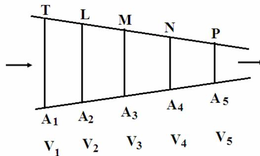
$$A_1 V_1 = A_2 V_2 = A_3 V_3 = A_4 V_4 = A_5 V_5 = \dots\dots\dots$$
