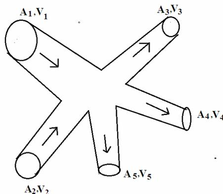
Here,  $A_1 V_1 + A_2 V_2 = A_3 V_3 + A_4 V_4 + A_5 V_5$
